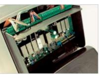
A safe system. In all of the versions, the control electronics are built-into the unit (except for version BK2200T) and is protected from environmental agents.
