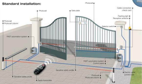
In the event a careful analysis of the automated gate's risks were to require it, the use of sensitive safety infrared or contact profiles becomes indispensable. If the gate leaves are of the panel kind, or in the presence of strong winds, the 230V version is SUGGESTED.
