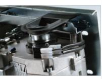
Precise, sturdy and dependable. FERNI features microswitches for adjusting the opening of the gate leaves and is made of long-wearing materials that do not require periodic maintenance.
