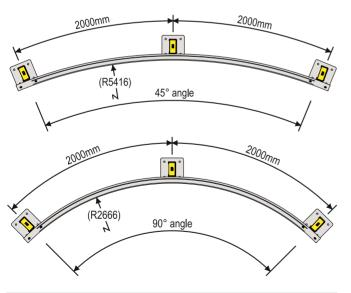
PART No.DESCRIPTION(Part Number is for rail only)WBR45IN550-GW-Beam rail 45 degree internal curve radius 550cm (26kgs) – HDGWBR90IN275-GW-Beam rail 90 degree internal curve radius 275cm (26kgs) – HDG
