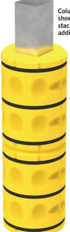
PART No. DESCRIPTION Column cushion kit, 610mm outer x CC610-200 200mm inner x 900mm high, 12kgs. Blow-moulded LLDPE with injected Shown above foam-filled core. Fits square: 150-200mm. Column cushion kit, 610mm outer x 250mm inner x 900mm high, 12.5kgs. CC610-250 Blow-moulded LLDPE with injected foam-filled core. Fits square: 200-250mm. Column cushion kit, 610mm outer x 300mm inner x 900mm high, 13kgs. CC610-300 Blow-moulded LLDPE with injected foam-filled core. Fits square: 250-300mm.
